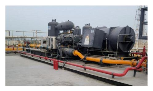
Our high-pressure and ultra-high-pressure gas injection compressor units.
