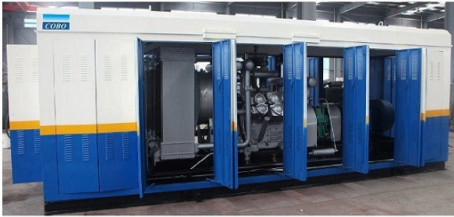
Our vehicle-mounted compressor unit.
