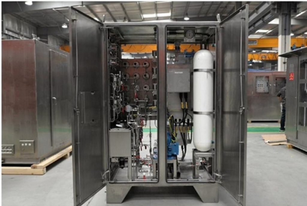
Our wellhead safety control system.
